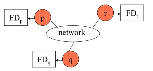
• A failure detector defined by a completeness property and an accuracy property
