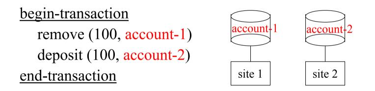
Crash during the transaction: rollback to the state before the beginning of the transaction
